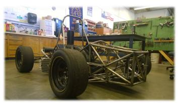
The car may look bare now but be warned, a full carbon and fiberglass body is in the process of being constructed right now! This will not only include body panels but a fully functioning undertray package to create downforce in highspeed corners while limiting the amount of weight and drag that might be found in a full aero package.
