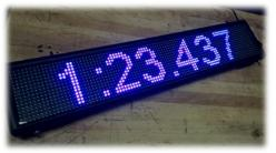
How does this benefit the team and the car? Prior to this lap timer, validation and testing of the car relied on human reactions. We have found that the most accurate team members are off by three tenths each lap. Relying on humans to time laps is inefficient, and when validating a design the most accurate data is necessary. The lap timer also helps train our drivers for competition. In 2013, the first four positions in autocross finished within a second of each other!
