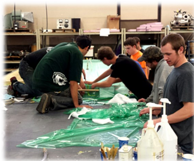
Undertray debulking in progress!
